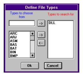
The left side of the dialog contains file types that you can specify or select. The right side shows the file types that are selected and will be used in the disk scan if you press the **Ok** button. In the case shown above, only DLL files will be scanned. To see what the controls in this dialog do, click on them with the mouse and additional information will be displayed.
